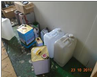
Photo of non-conformity NC-missing secondary containment.JPG
